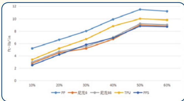
长玻纤增强多种塑料基材冲击性能对比 Comparison of impact property of various plastic substrates with long glass fiber
